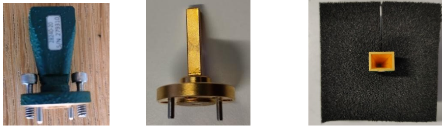
Figure 1: The Standard Gain Horn (SGH) antenna and open-ended-waveguide (OEWG) antenna we used for measurements in the frequency range 90 GHz to 140 GHz.
