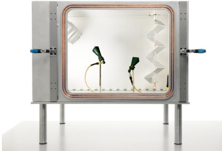
Figure 15: Example of a mm-wave RC chamber in development in TU/e
